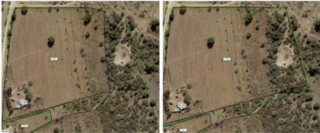
Figure 21: Incorrect use of orthophoto (left) and correct use (right) based on field data capture
