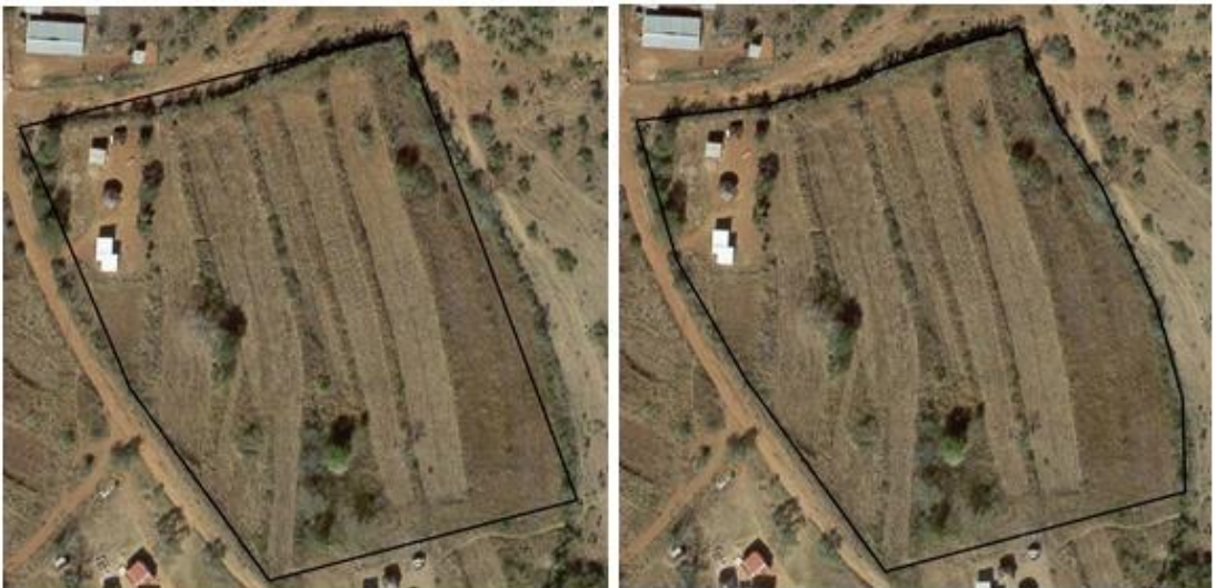
Figure 27: Edit example - incorrect (left) too few vertices, correct (right) better fit to ortho
