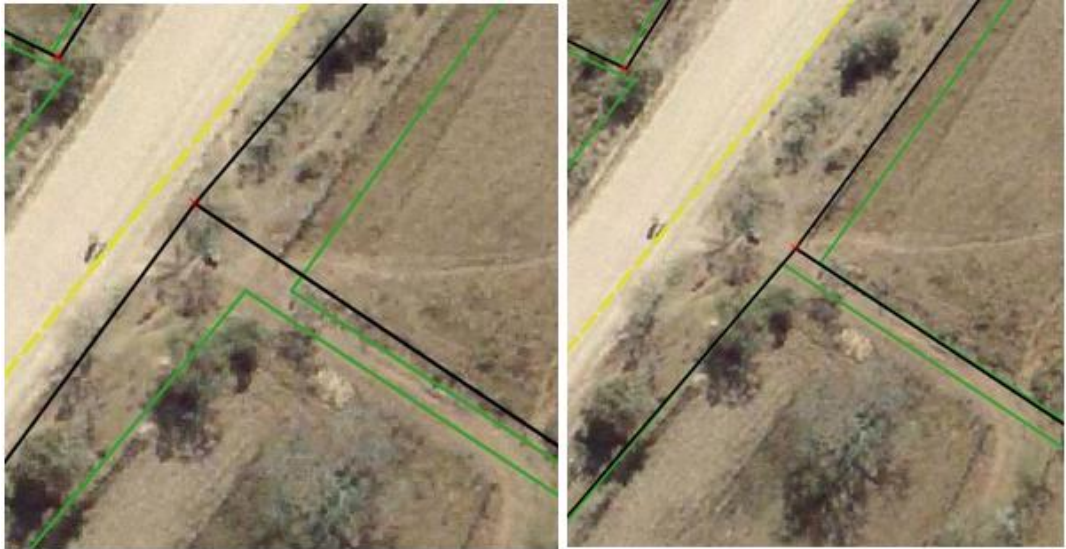
Figure 23: Edit example - incorrect (left), correct (right)
