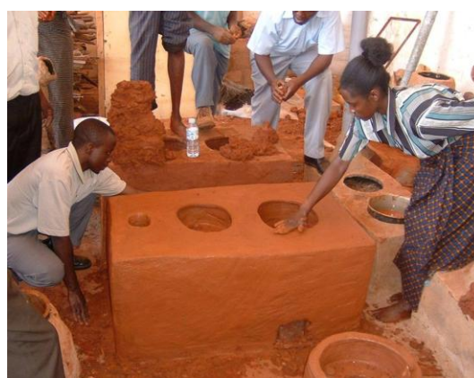
Figure 10 – PAMENU, Uganda – Preparing Domestic Charcoal Stoves
