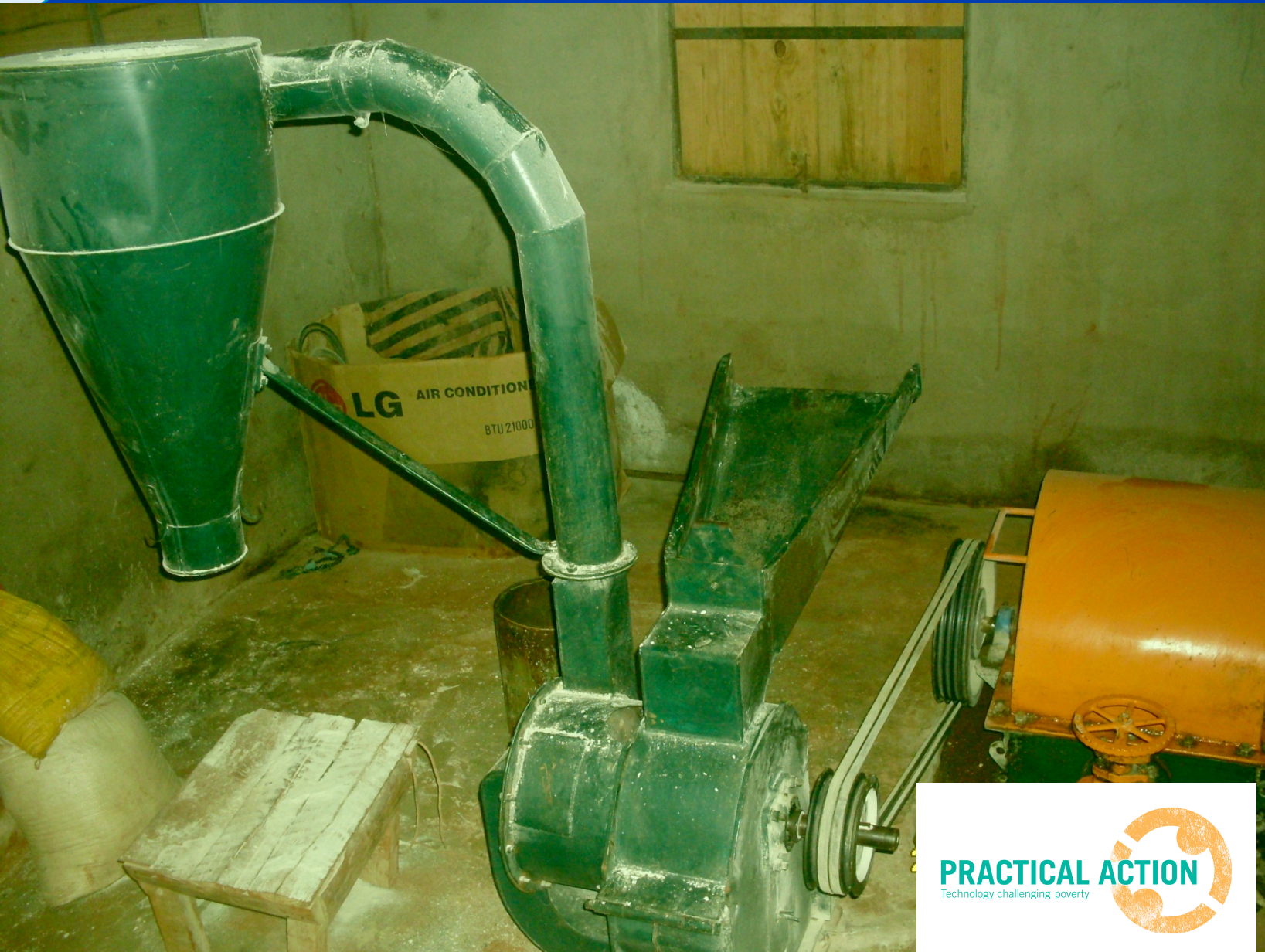
Hydro mechanically powered grinding mill at Ndiriri, Manica.
