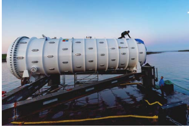
Figure 10.12. Microsoft Project Natick Phase 2—modular submersed server with renewable ocean energy and ocean cooling, Scotland. Photo by Scott Eklund/Red Box Pictures
