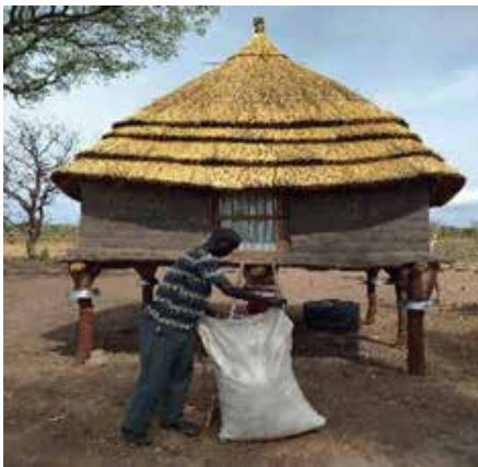
Figure 13: Traditional grain storage stores with rat deterrence
