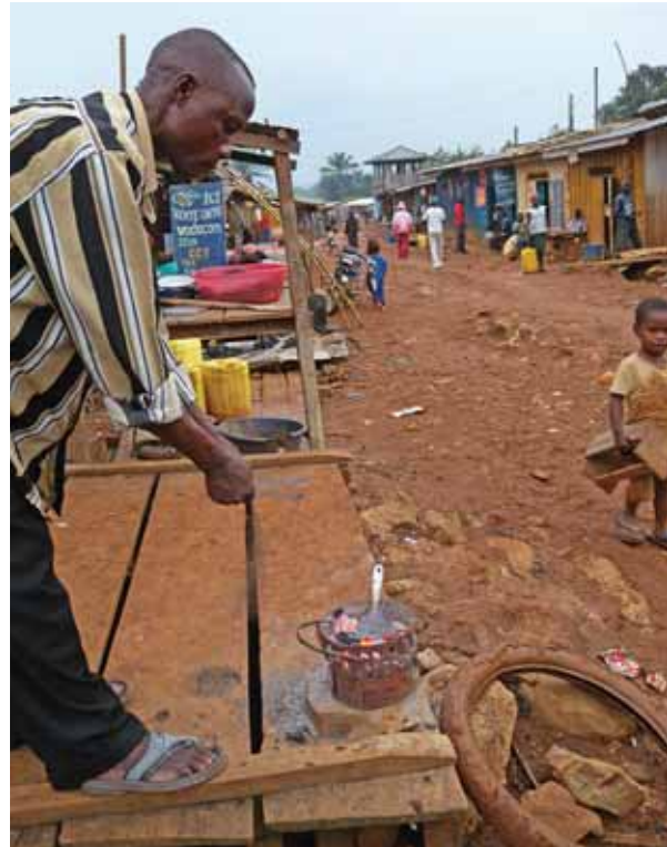
A gold dealer heats a clump of mercury containing gold amalgam on the roadside beside his shop. As the burning is done in the open air, toxic mercury vapours spill directly on streets crowded with people and children
