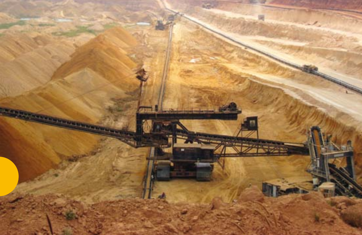
Open-cast mining of phosphate rock in Togo. Most of the world's phosphate rock is extracted from open pits, as shown here, or from large-scale mines equipped with drag lines or shovel/excavator systems. Credit: Alexandra Pugachevsky
