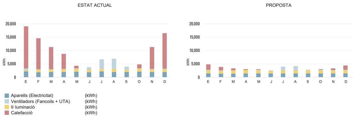
Figure 24. Energy demand of AMB Headquarters before and after the renovation. Image provided by AMB.
