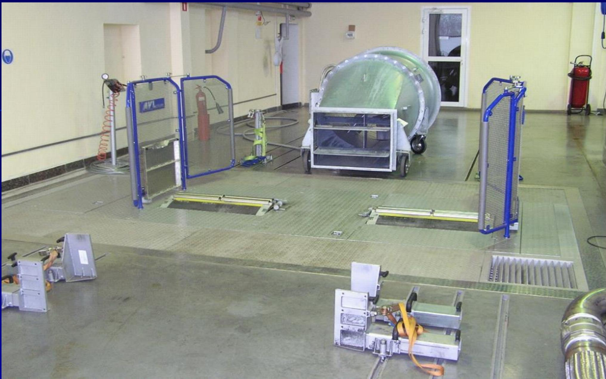
Modern chassis dynamometer (vehicle test bench) of AVL Company (model RPL1220/12C23M17/APM150) installed in Kyiv, Ukraine to test road vehicle on driving cycles
