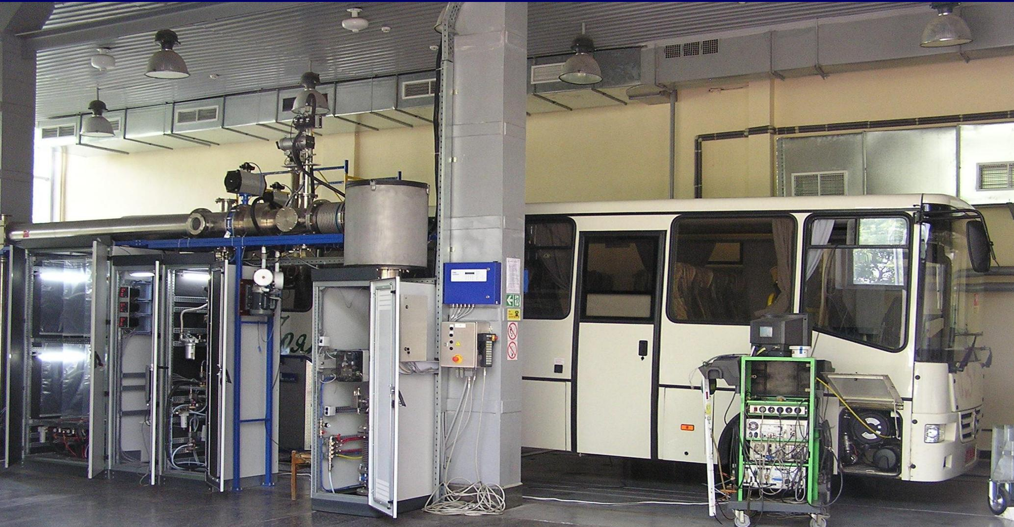
**Investigation of exhaust emission of bus (R&D) on chassis dynamometer (real driving conditions reproduction). Ukrainian EMMS-CVS-010 system on the left.**
