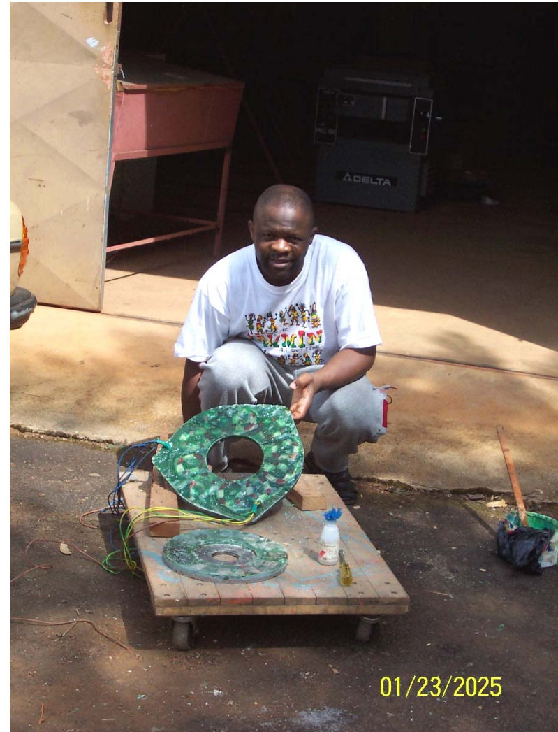
Casted stator is ready for mounting
