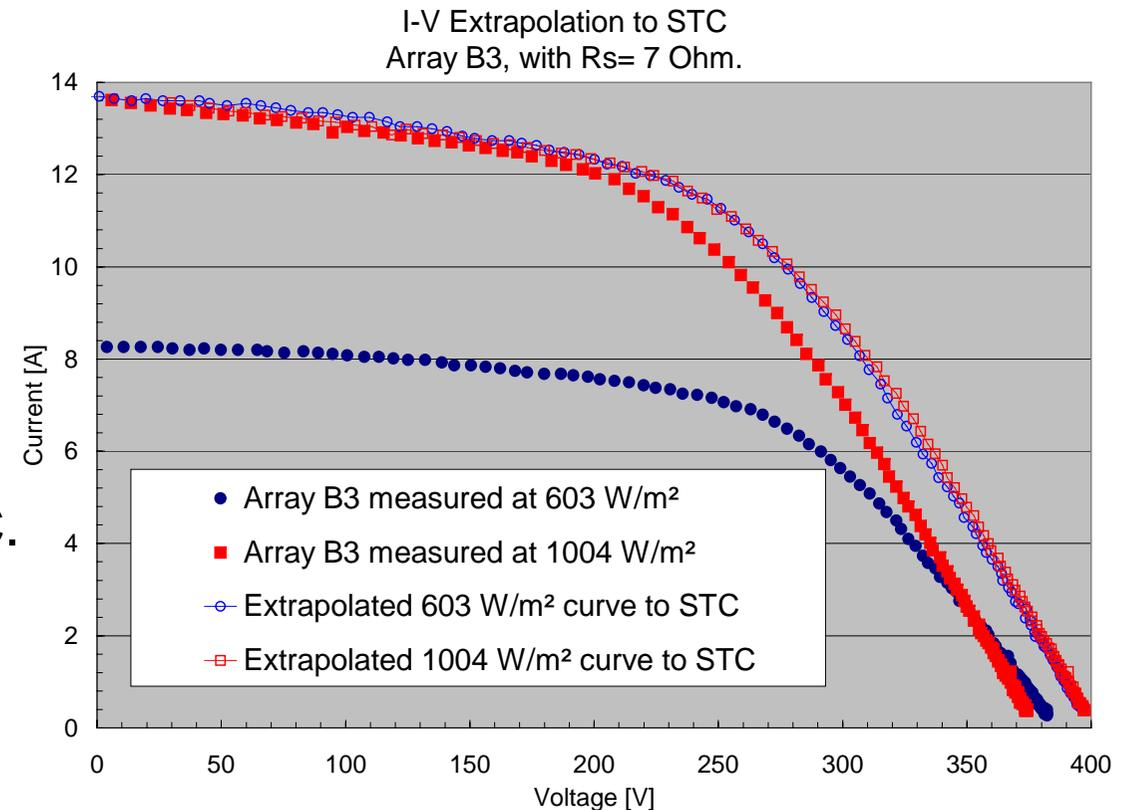
The extrapolated  $P_{\max\_STC}$  of both scans with a value of  $R_s = 7$  Ohm resulted in a 2828 W (603 W/m<sup>2</sup> scan1) and 2832 W (1004 W/m<sup>2</sup> scan2)
