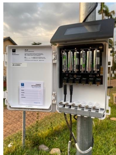
Projet Horticulture Ghana- Technology: better manage water and other inputs by measuring air temperature, humidity, rainfall, soil temperature and moisture.
