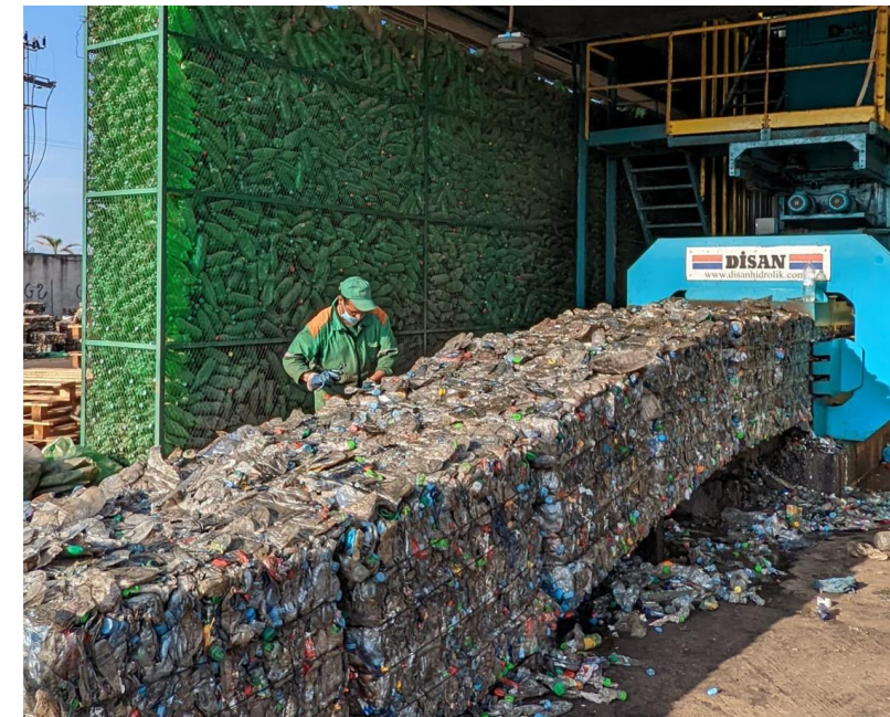
Plastic baler at a sorting centre in Oum Azza, Morocco. Photo: SWITCH2CE
