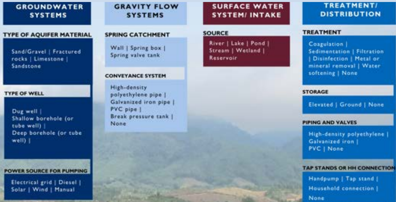
Figure 2. Varied characteristics of rural water supplies in low- and middle-income countries (Source:Vanessa Guenther, Aquaya Institute). These aspects may be used separately or in combination, typically with an emphasis on simplified engineering to fit local conditions.
