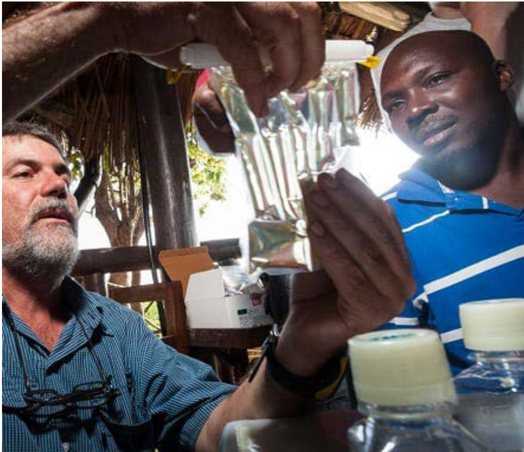
Figure 21. Water sample added to an Aquagenx compartment bag (Source: Engineering for Change)
