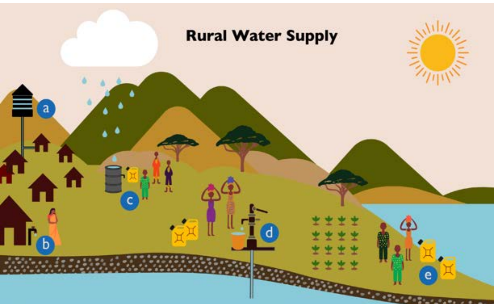
Figure 1. Simplified diagram depicting several common rural water supply methods in low-income settings, including (a) piped household connections, (b) public tap stands, (c) household rainwater harvesting, (d) community groundwater boreholes with handpumps, and (e) surface water collection (Source: Vanessa Guenther, Aquaya Institute)
