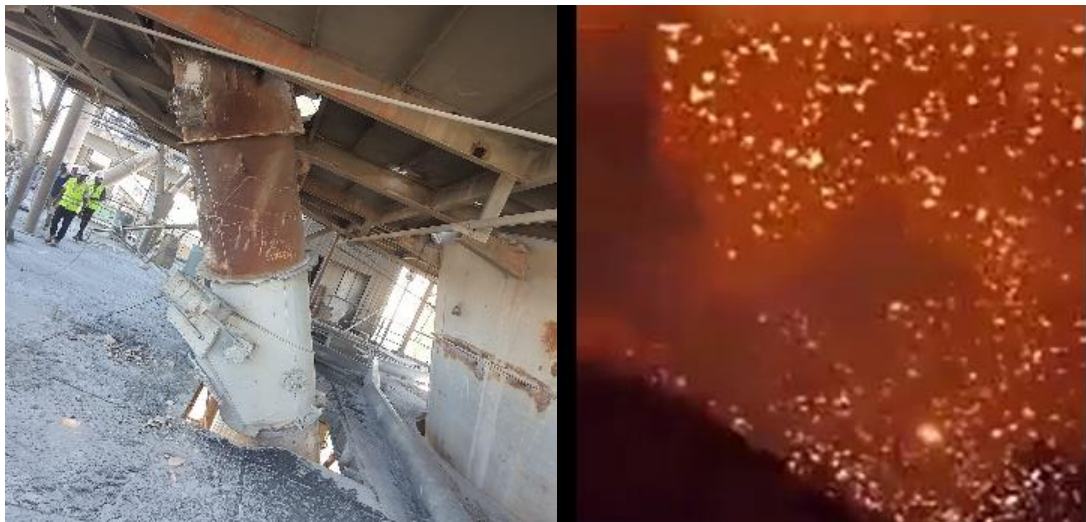
Bottom cyclone hot meal pipe and sparks
