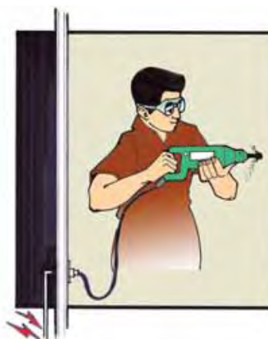
Figure 28: All electrical equipment should be earthed correctly. An independent earthing rod should be used to connect earthing wires from machines.
