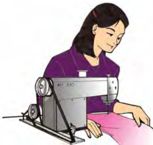
Figure 18: Attach covers to moving parts of machines. Design them not to be obstacles to your work.
