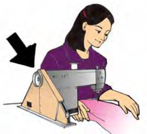
Figure 18: Attach covers to moving parts of machines. Design them not to be obstacles to your work.
