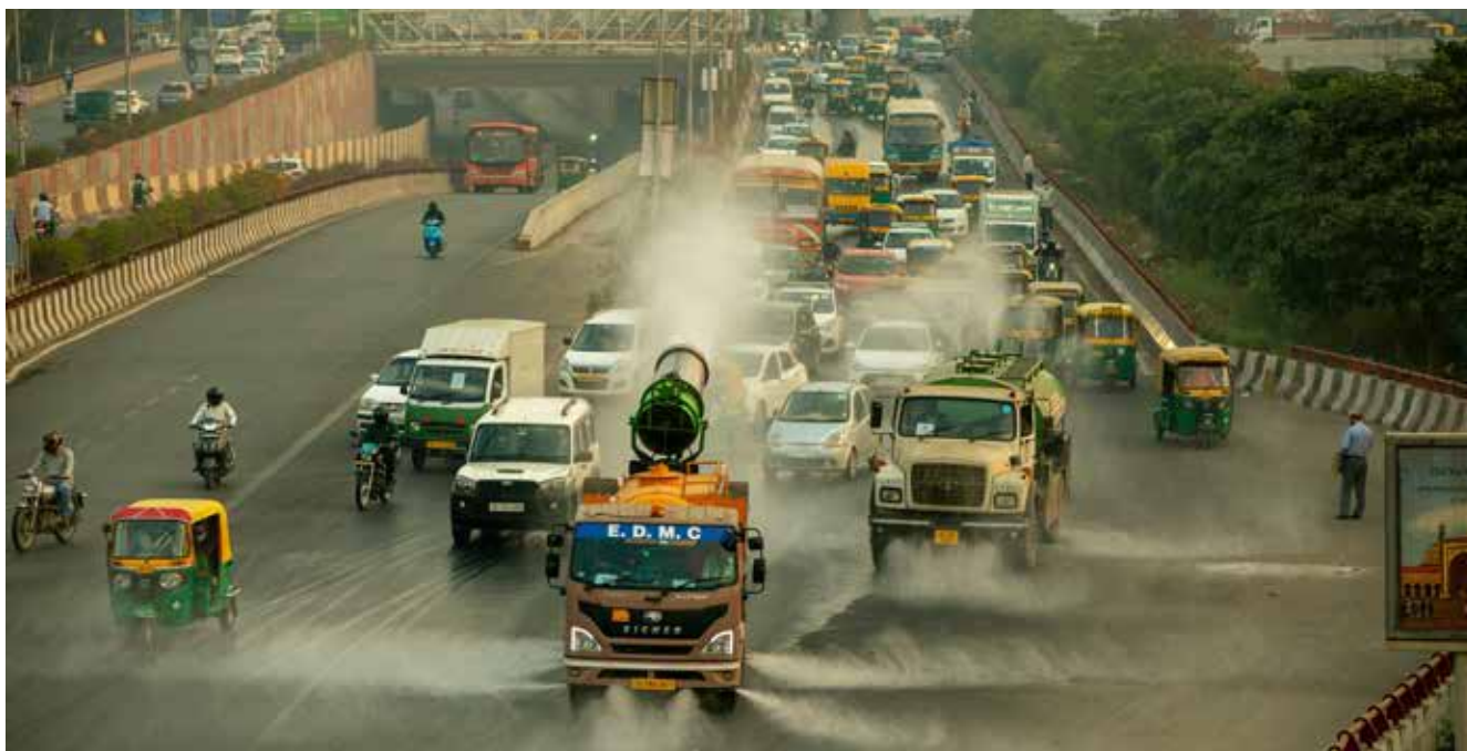
A municipal truck uses anti smog gun to spray water on the road for dust suppression to reduce air pollution in Delhi, India. © Shutterstock
