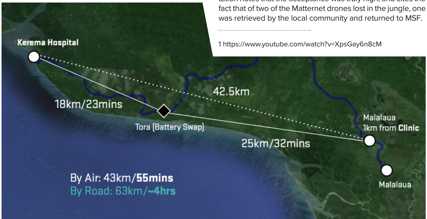
Figure 2 Aerial transportation routes between Kerema hospital and Malalaua. The aerial distance between the two points is 42.5 km. In order to swap batteries midway, Matternet first flew the drone to Tora, and then on to Malalaua. These two flights took about 55 minutes in total (including the time for battery swap). In contrast, driving a car between the hospital and Malalaua takes approximately four hours. Credit: Matternet.
