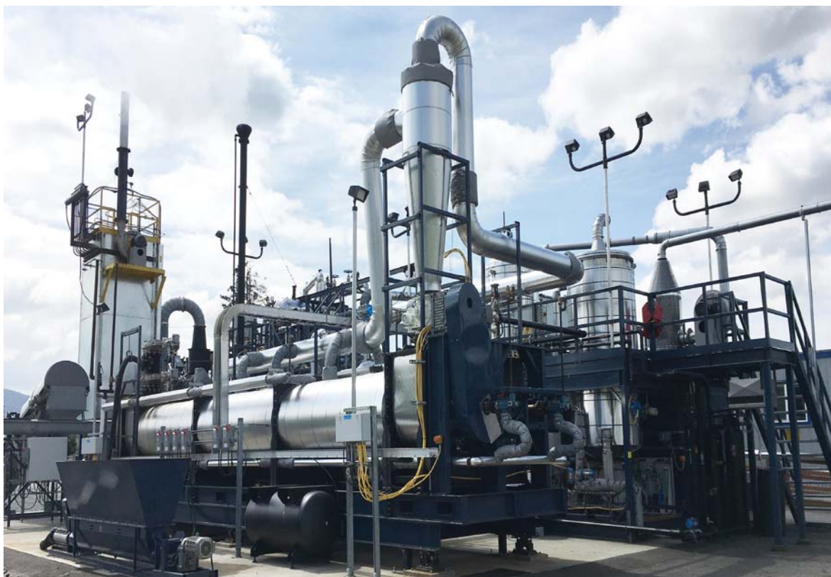
A combined heat and power plant that recovers energy (heat and electricity), potable water and ash from faecal sludge and other combustible waste. Photo: Flickr / SuSanA Secretariat / Janicki Bioenergy
