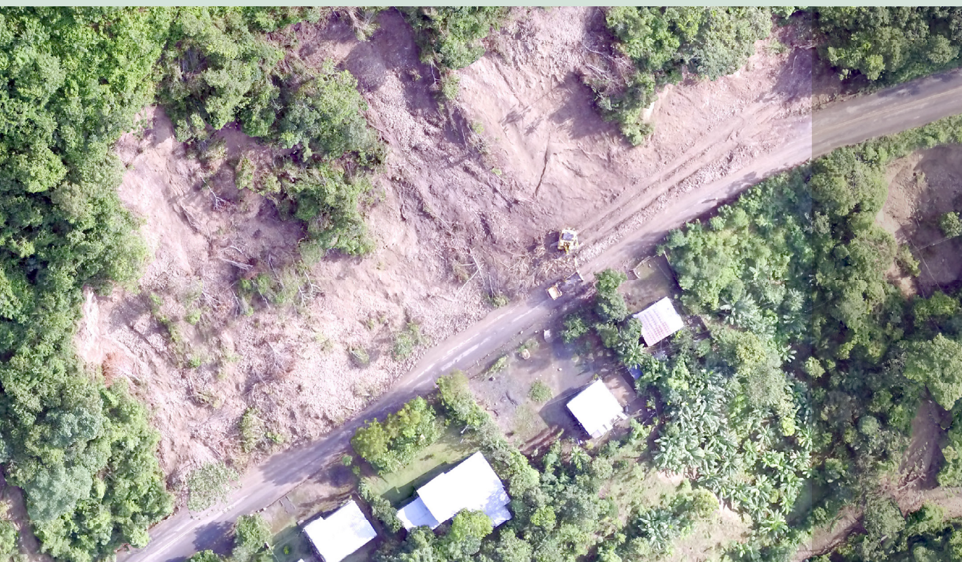
Figure 1 A landslide in St Isidro, Manabí province caused damage to roadways following the earthquake. Image: Francisco Ruiz, April 2016.
