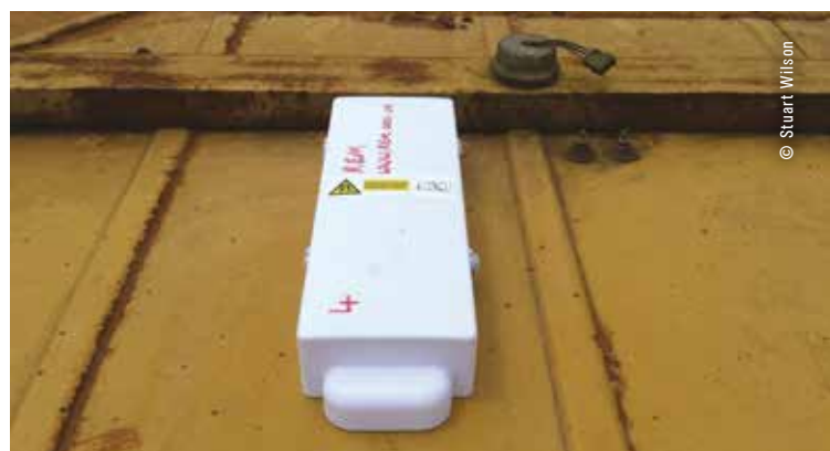
Photo 14 GPS box fixed to the roof of a machine
