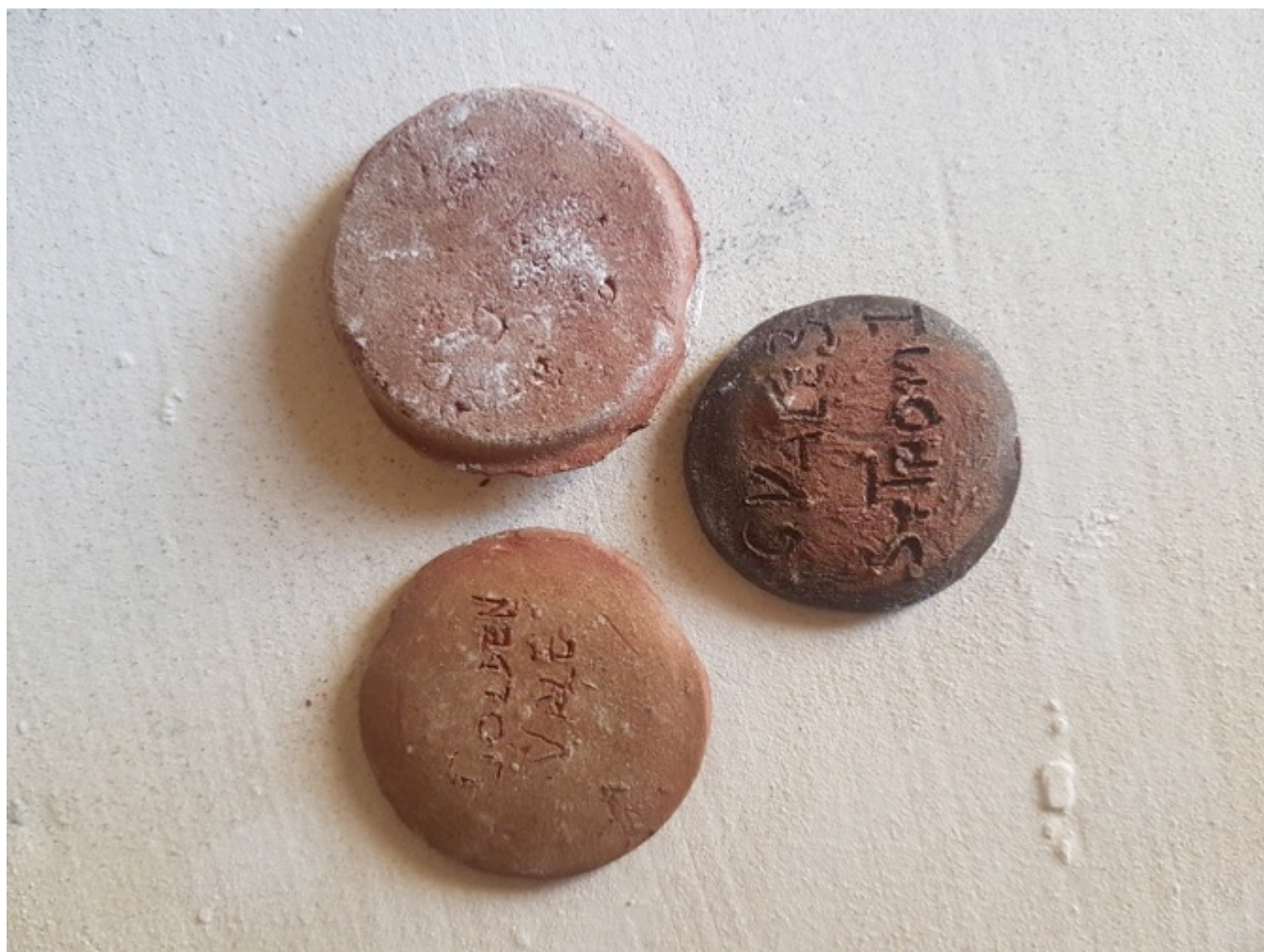
Figure 2: Golden Vale clay body testing [slip, throwing clay, Golden Vale + St. Thomas mix]
