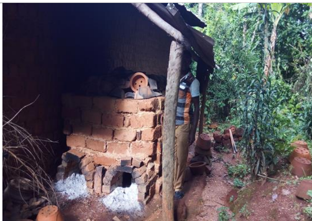
Fig 9: Traditional Kiln for the drying of clay products
