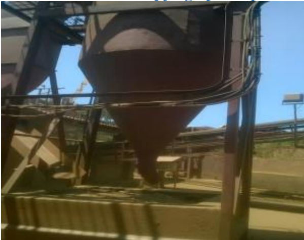
Dust-water trapping mechanism
