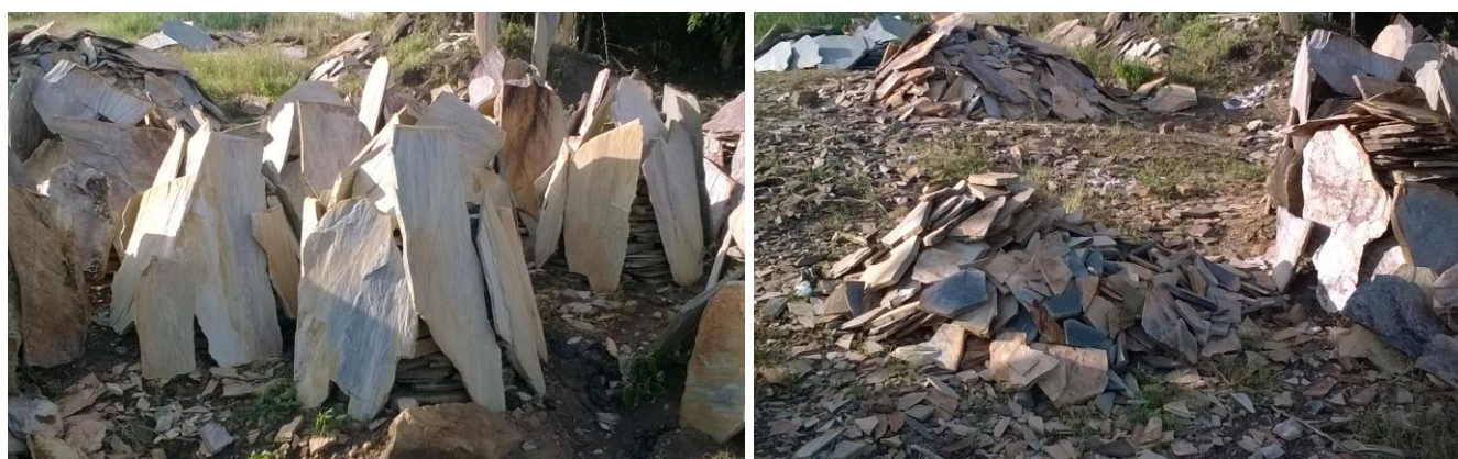
Figure 2.7: Some limestone sources along Aburi Mountains, Eastern Region used for wall facing and floor paving. Each of the rock groupings cost GH¢250 or US$65.80 (Source: field survey, 2016).
