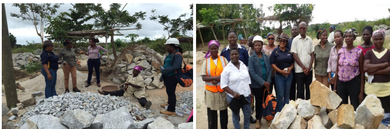
Figure 2.9: Granitic rocks being crushed for construction materials by quarry women at Esuakyir, Central Region. Cost is GH¢1000 or US$263.16 per truck (Source: Women in Mining fieldwork, 2015).
