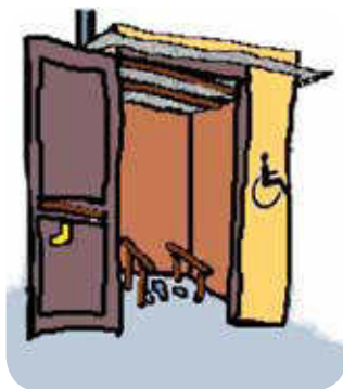
Adapted latrine with handrails
